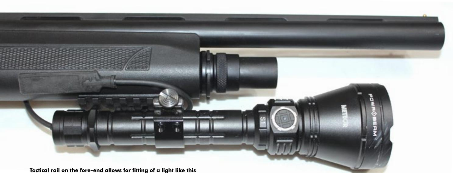
Tactical rail on the fore-end allows for fitting of a light like this Powa Beam unit with tape switch for activation.
