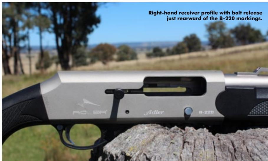
Right-hand receiver profile with bolt release just rearward of the B-220 markings.
