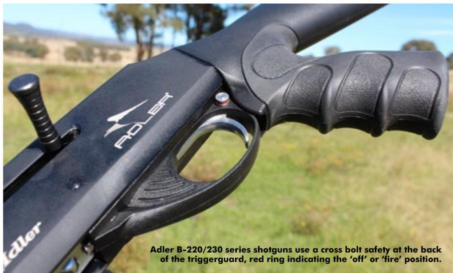
Adler B-220/230 series shotguns use a cross bolt safety at the back of the triggerguard, red ring indicating the 'off' or 'fire' position.
